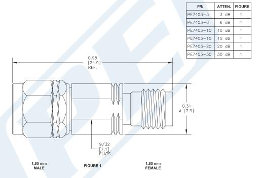
6 dB Fixed Attenuator, 1.85mm Male To 1.85mm Female Passivated Stainless Steel Body Rated To 1 Watt Up To 65 GHz from Pasternack Enterprises has same day shipment for domestic and International orders. Our RF, microwave and millimeter wave products maintain a 99% availability and are part of the broadest selection in the industry.
